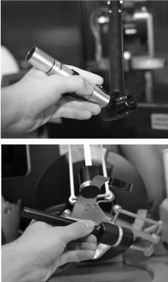
**Figure 1:** Two common haptic interface devices. Both can read position and output a force. Sensable Phantom 1.5 (above) can also output rotational forces. Force-Dimension Omega 3 (below) could arguably still have higher desire factor.
